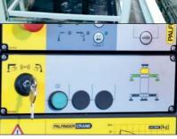
\* ISC or an alternative system for monitoring stability is mandatory in the version compliant with EN12999:2009.
