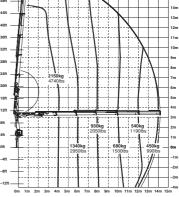
The outreaches stated are with a boom angle of 20° and are therefore not the maximum.
